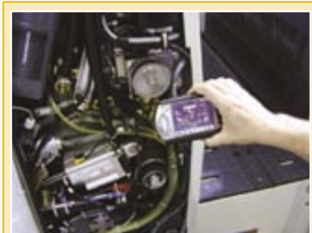
Eye see you. MAN Roland's E-Eyes gives MAN Roland's RRT technicians the vision to repair a press via remote control.
